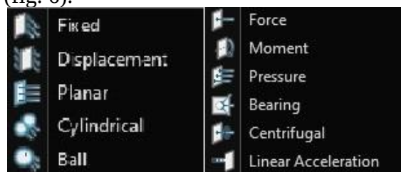
Fig. 6 Generative Design constraints and loads toolbar
