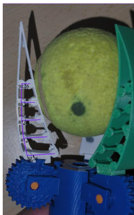
Fig. 7. PP finray finger with rib angles measurements
