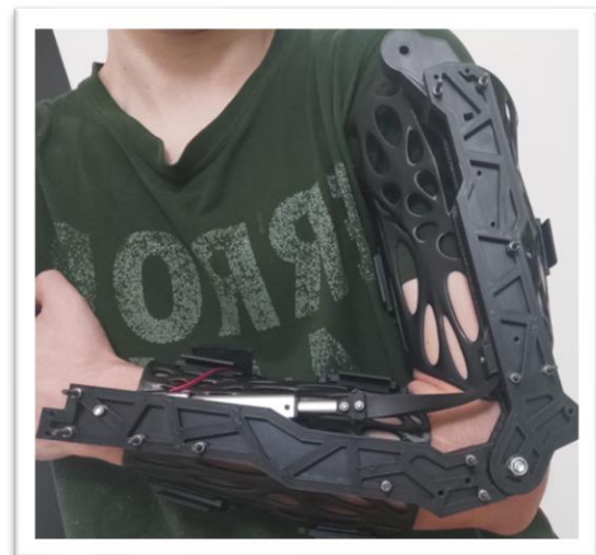
Fig. 6. Skeleton Ensuring Correct Relative Motion of the Two Modules Fig. 7. Prototype or robotic orthosis
