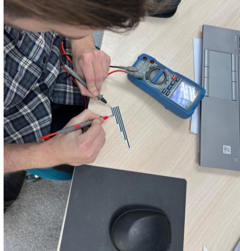
Fig.3. Samples conductivity measurement process
