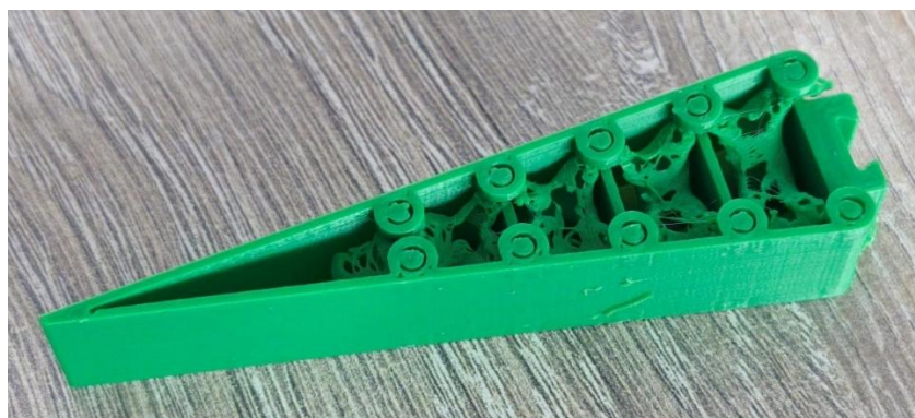
Fig. 2. Finger 3D-printed in PLA with support structure
