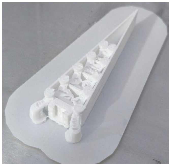
Fig. 4. Finger 3D-printed in PP with support structure and Raft support
