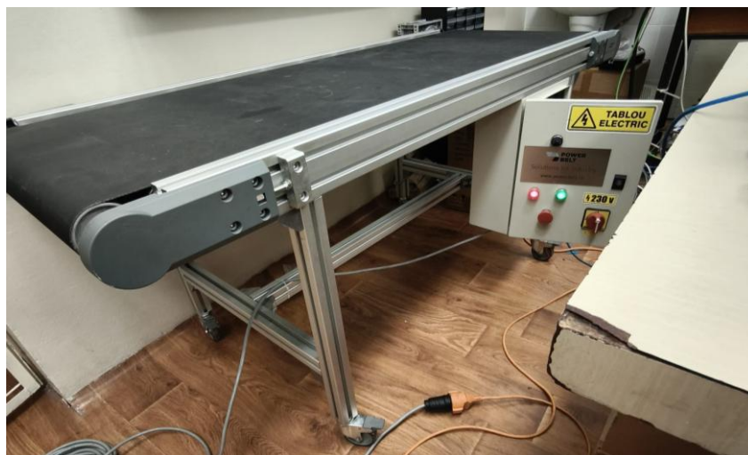
Fig. 6. Power Belt Conveyor
