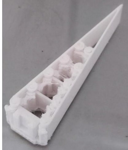
Fig. 3. Finger 3D-printed in PETG with support structure
