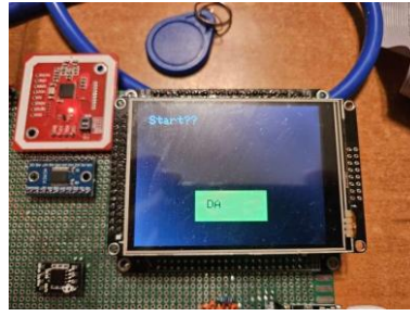
Fig. 6. TFT screen connected and functional.
