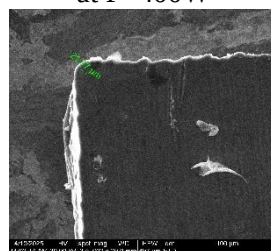
Fig. 22 Outer corner radius at P=400W
