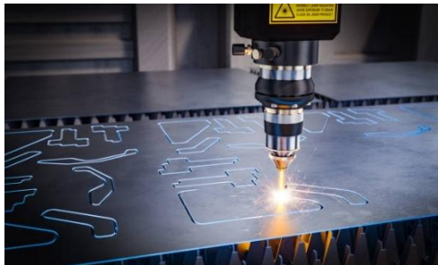
Fig. 1. Complex shapes produced using laser contour cutting technology [2]
