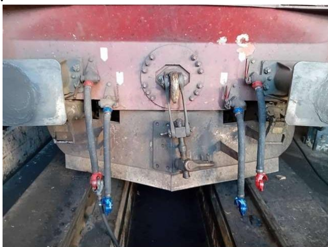
Fig. 1 Coupling attached to locomotive
