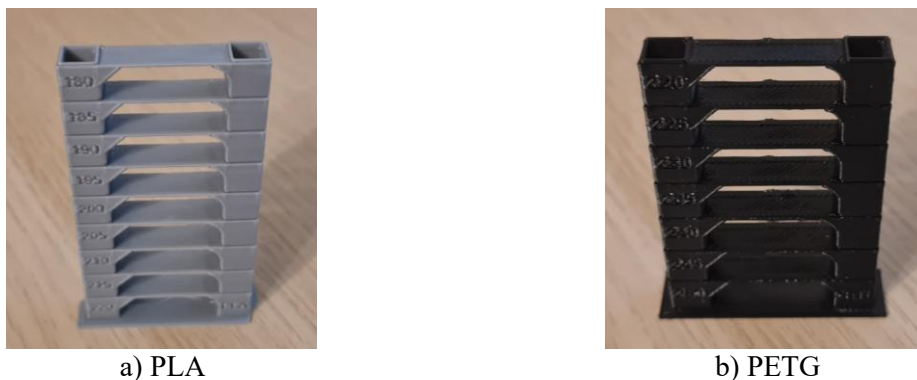
Fig. 2 – Samples tested by varying the temperature of the two materials:
