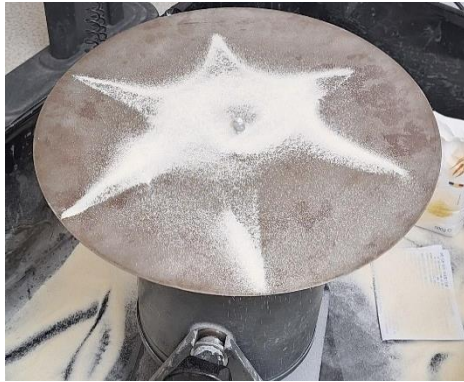
Fig. 2 Shaker with circular plate, resonating at 181 Hz
