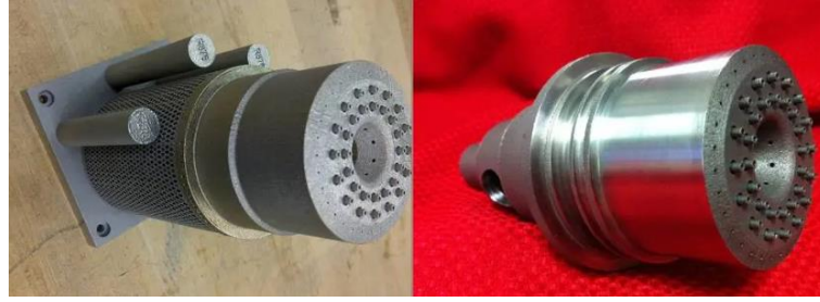
Figure 1 "Injector made with the help of a 3D printer"
