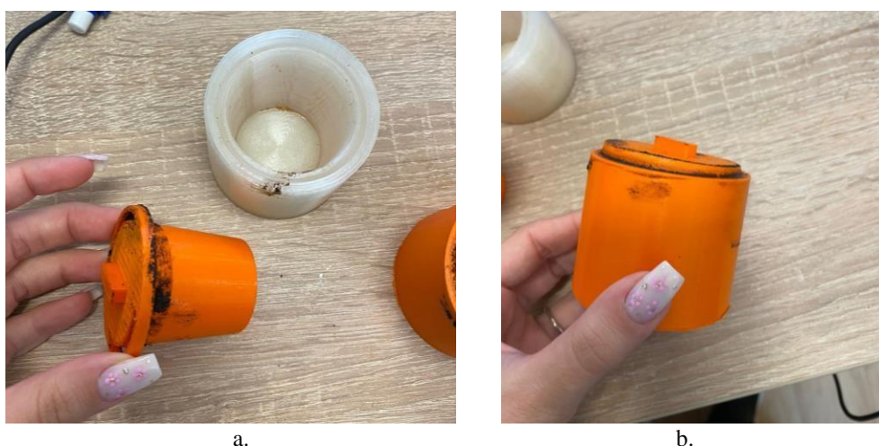
Fig. 2. Molds used in the production of coffee grounds containers; a - mold before use, b - mold destroyed by sticking of the composition to its walls.
