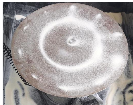
Fig. 3 Chladni pattern of a resonating plate, at 401 Hz
