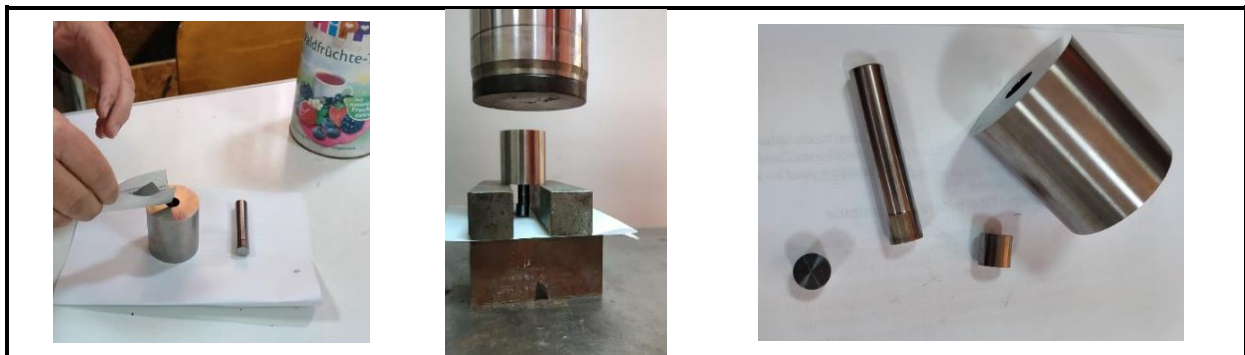
Fig. 3. Making the piece by pressing the metal powder with a 100t press
