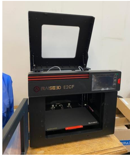
Fig.3. The 3D printer used in creating the mold for producing coffee ground containers.
