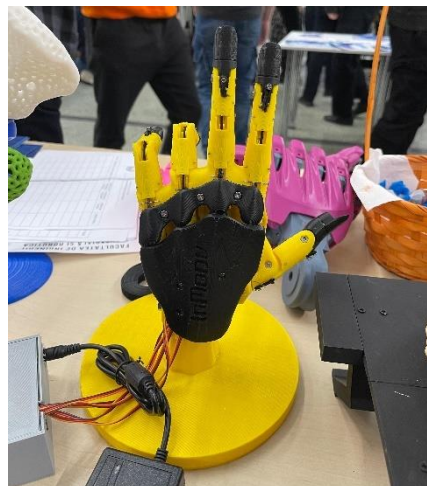
Figure 2 "3D Printed Robotic Hand Controlled with Arduino"
