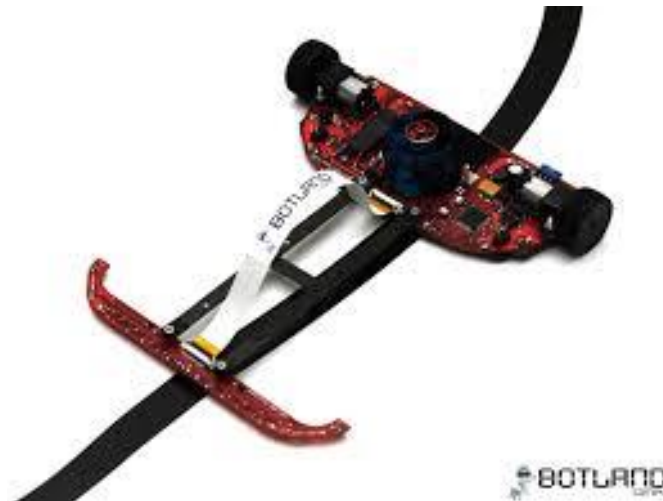
Fig 3. Example of a Line Follower robot equipped with a prebuilt EDF
