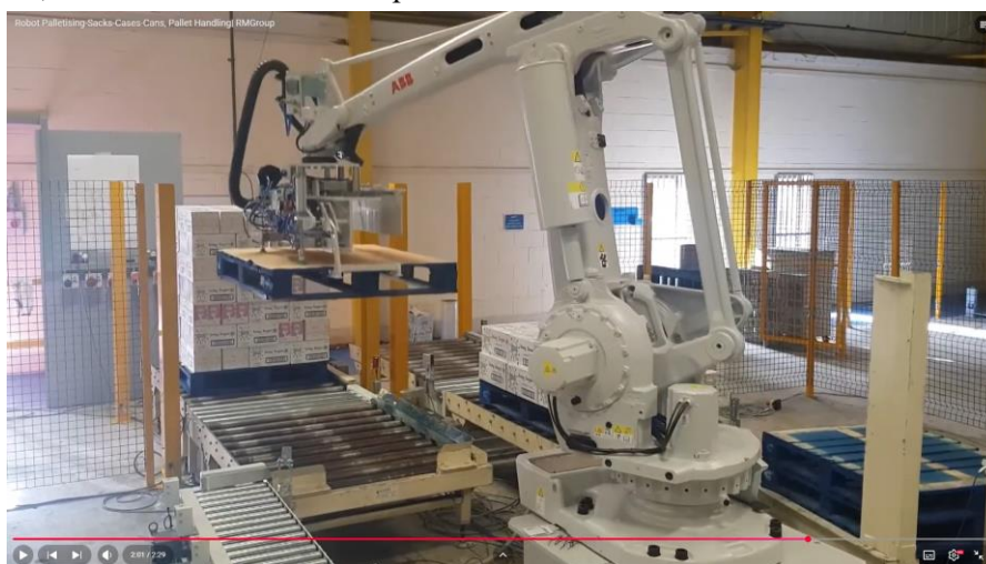
Fig. 1. Reference model for the robotic palletizing application
