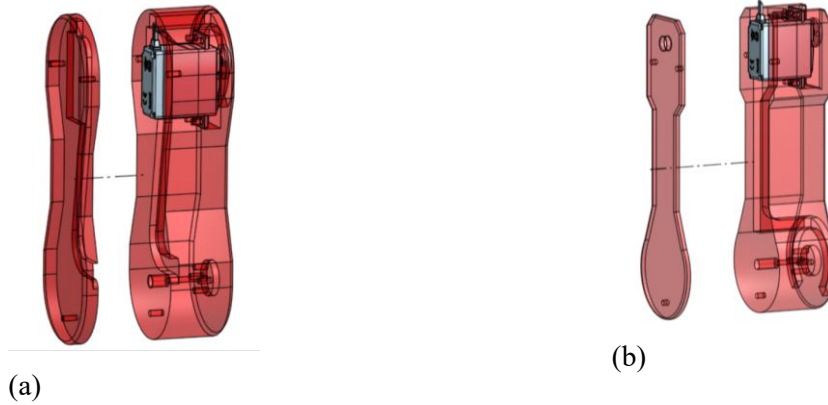
Fig. 6. Arm Segments a) Proximal arm segment; b) Distal arm segment
