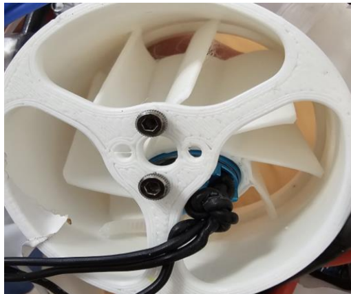
Fig. 10 heat based failure of the turbine
