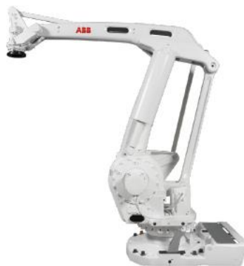
Fig. 2. ABB IRB 660 industrial robot used for palletizing
