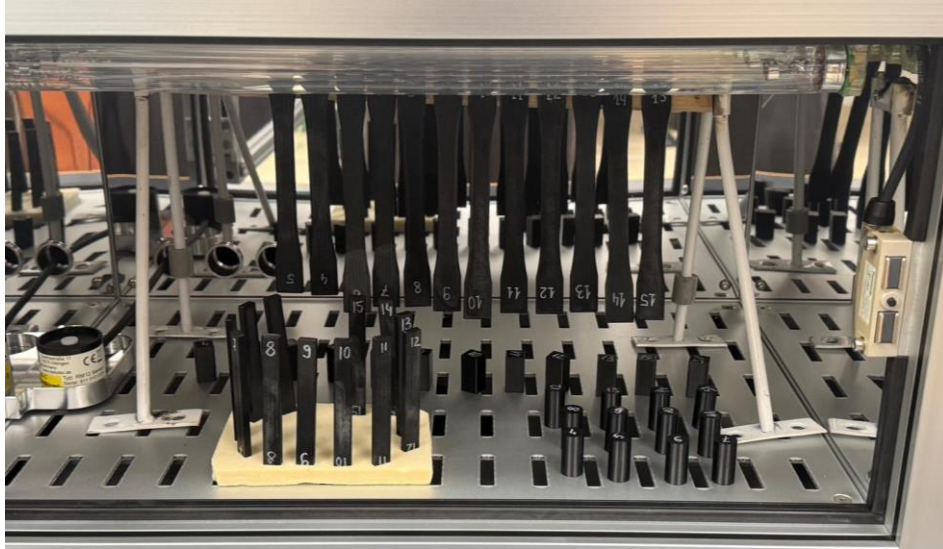
Figure 2. Specimens exposed to UV in the irradiation chamber
