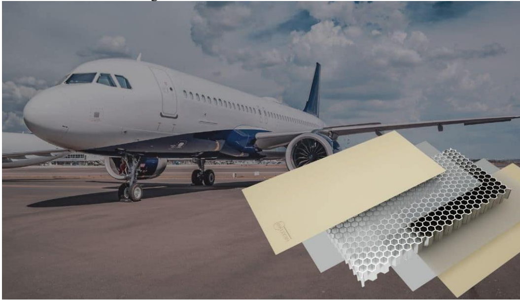
Fig. 8 Exploded view of a sandwich-type structure
