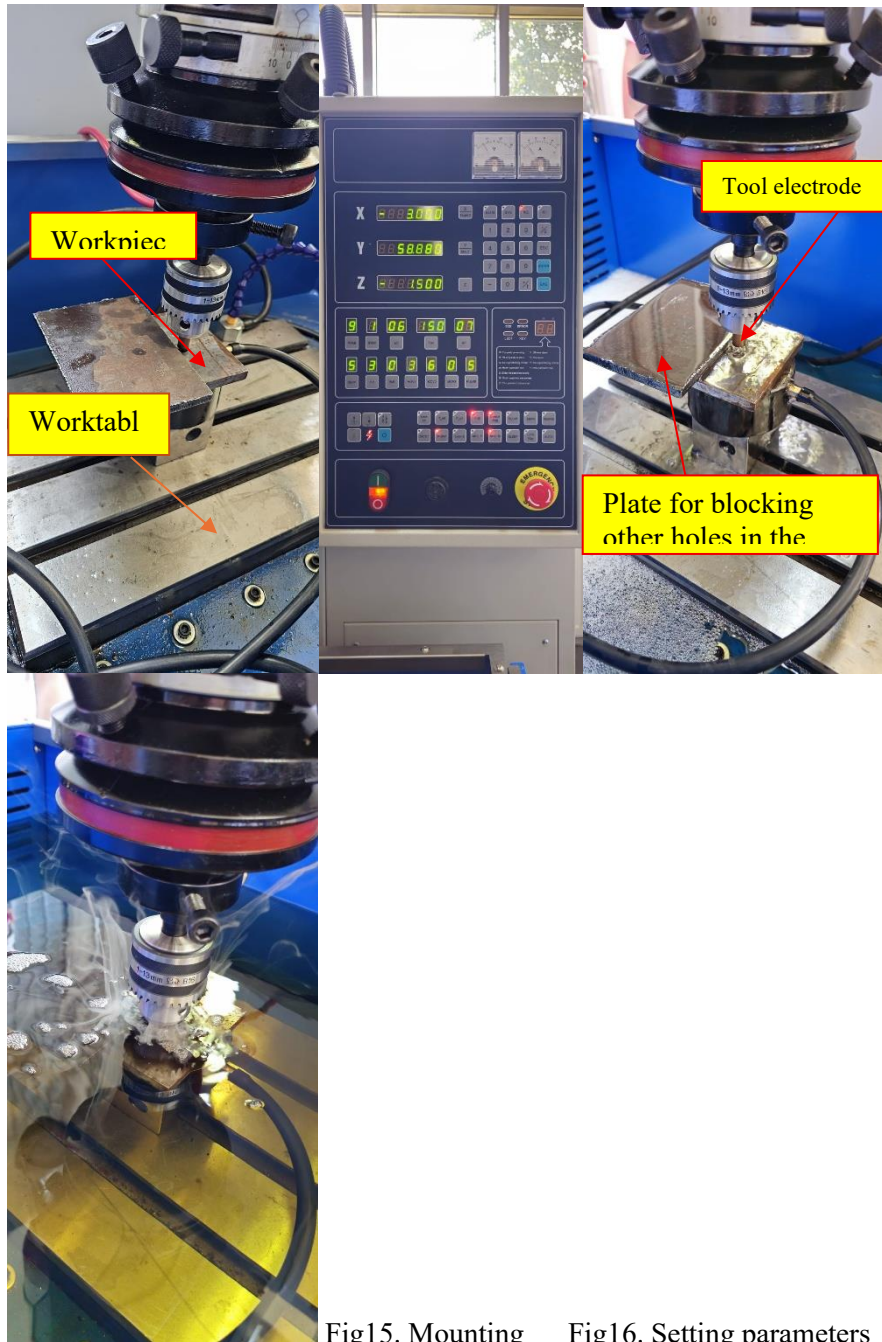
Fig15. Mounting Fig16. Setting parameters Fig17. Starting dielectric Fig18. Machining
