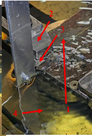
Fig. 2. Wire EDM cutting process using a device mounted on the EDM machine
