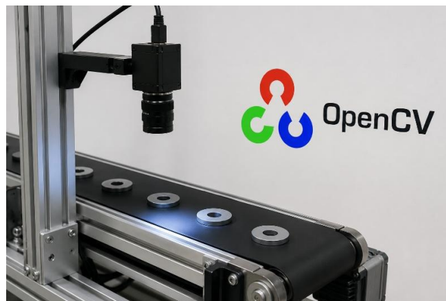
Fig. 3. Recognition subsystem used for image-based inspection [9]
