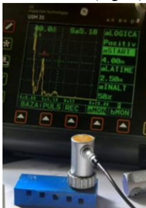
Fig.15: More attenuated signal than in the previous specimen
