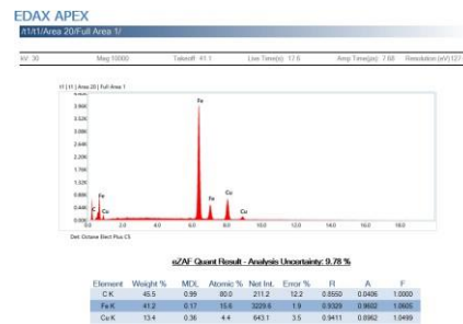
Fig. 6 EDX analysis of the electrode before EDM Fig. 7 EDX analysis of the electrode after EDM
