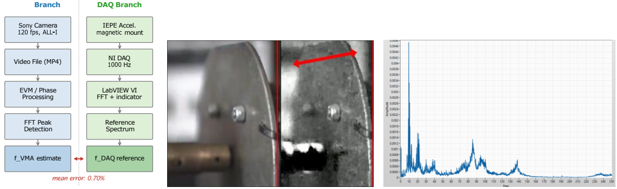
Figure 1. Fig. 1. (a) Dual acquisition chain (VMA + NI DAQ). (b) Original vs. VMA-amplified frame; arrow marks detected motion on flange face. (c) LabVIEW FFT with peak at 10 Hz.
