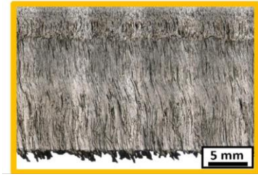
Fig. 9. Surface roughness in plasma cutting [21]
