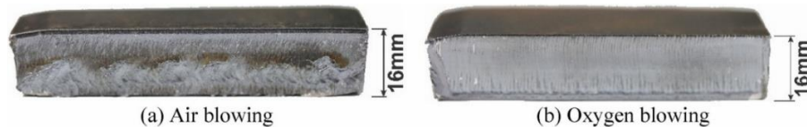
Fig. 7. Surface roughness in laser cutting using air or oxygen assist gases [22]
