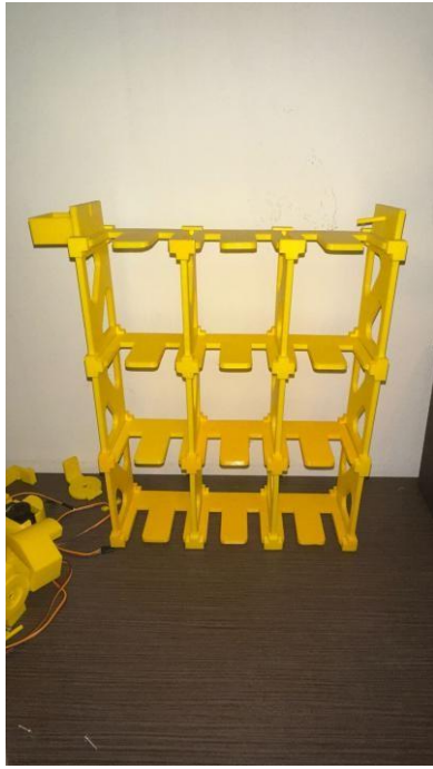
Fig. 6. Printed PLA storage cabinet assembled prototype
