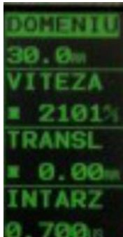
Fig.8: Flaw detector settings
