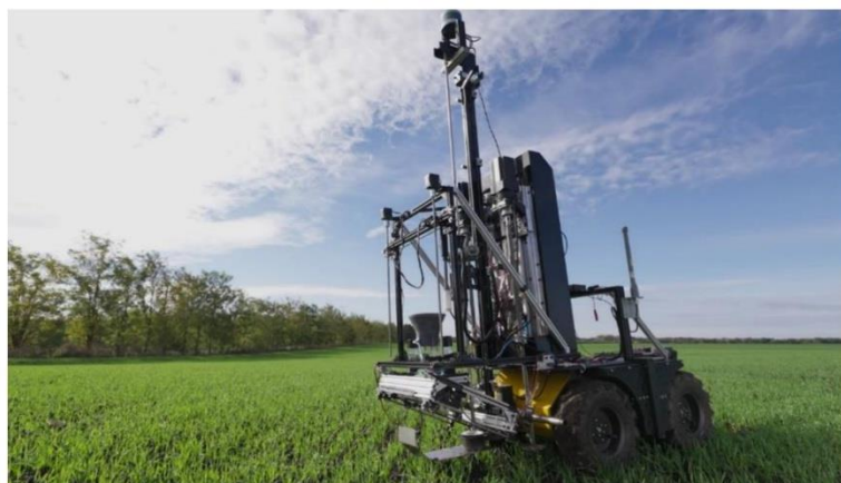
Fig.1.5. Autonomous robot for soil sampling and analysis – Agrobot Lala [2]
